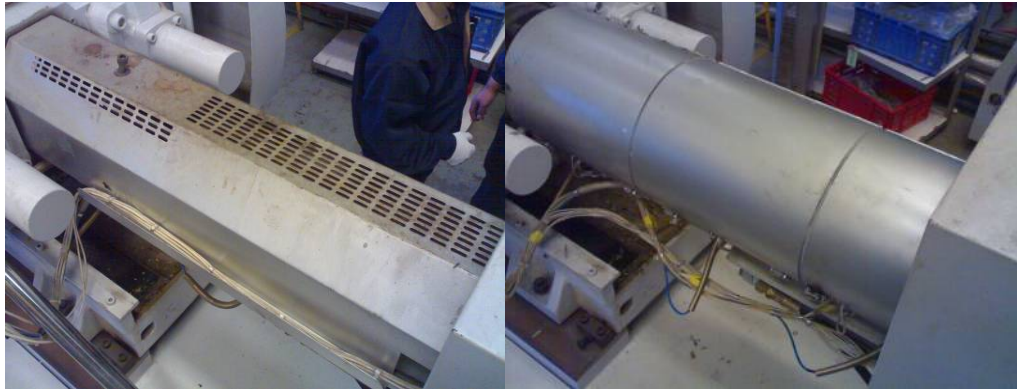
Figure 5-3: Before and after upgrading using infrared energy-saving heater band
