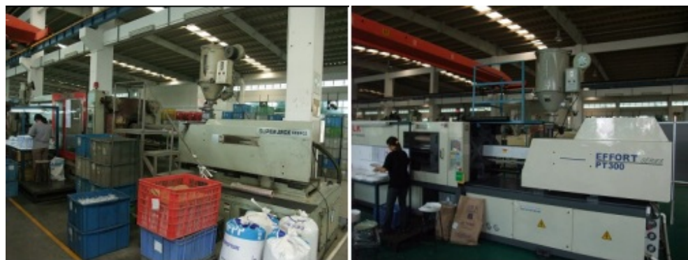
Figure 5-6: Conventional injection-molding machine vs. direct pressure injection molder with servo system
