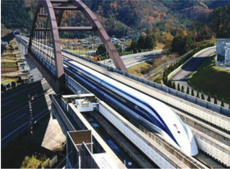
FIGURE 5.12 The Japanese MLX01 MagLev Experimental Train.
